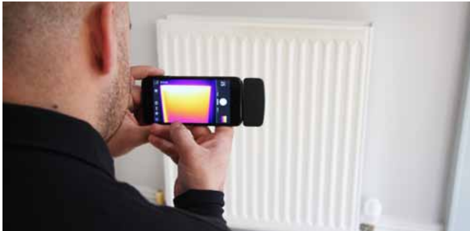
Using a heat detection camera we identify the inefficiency of each radiator before a flushing, and see the heat efficiency improvements after the flushing
