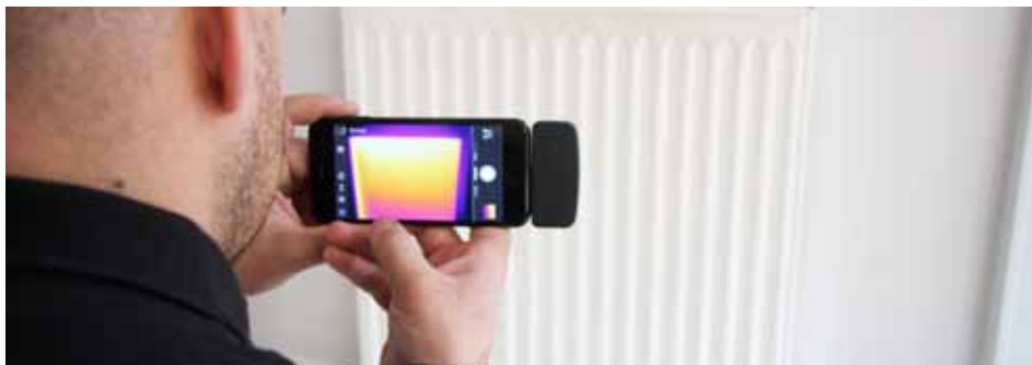
Using a heat detection camera we identify the inefficiency of each radiator before a flushing, and see the heat efficiency improvements after the flushing
